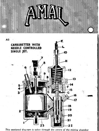
This sectioned diagram is taken through the centre of the mixing chamber and float chamber, showing the float and jet and throttle mechanism. The float and needle are shown as one piece as for types 259 and 261, but in type 223 the float needle (1) is separate from the float (2), but is attached thereto by a spring bow fastened to the float at the place marked (E). The cable (K) and its anchoring (K1) are diagrammatic as in practice the cable anchoring is in front of the jet.
