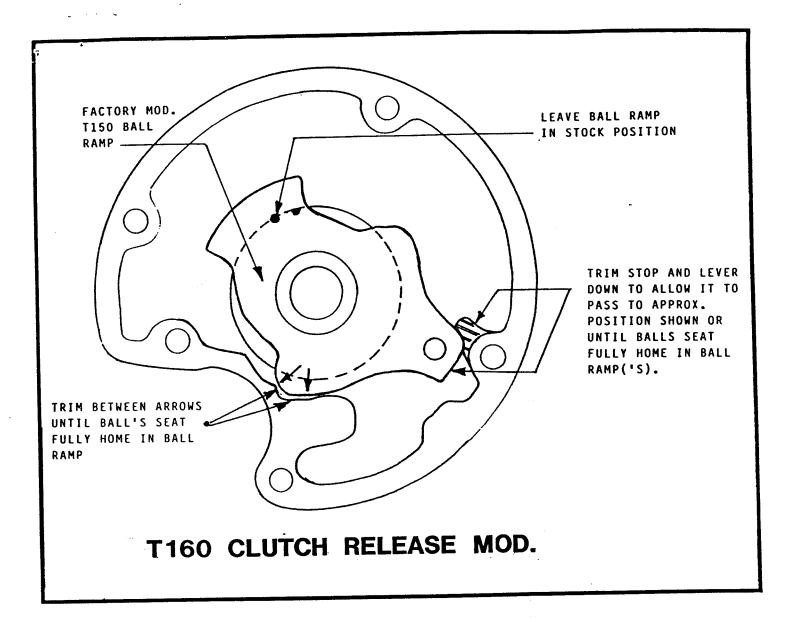
Additionally, on the T150, the "ball-ramp" in the primary cover will have to be removed. Heat the case to 150 degrees F. (hot water) and press it out. Then a new groove will have to be machined, 15 degrees counter clockwise to the old one. The ball ramp is hardened and you will have to grind, with a small wheel, a new groove. The T160 the ball ramp can be left in the stock position. Heat the T150 case again and replace the ramp utilizing the new groove.
