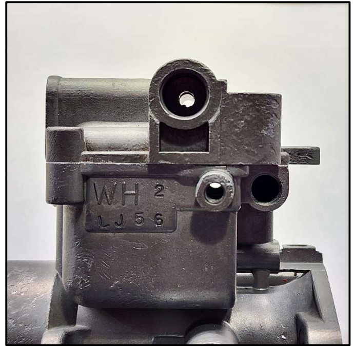
Figure 14 – The float chamber cover is placed onto the carburetor body to confirm fit. Unlike figure 6, there is no gap present, ensuring a proper fit of the gasket, reducing any chance of a fuel leak.
