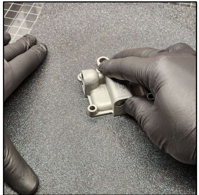
Figure 8 – With the coarse emery cloth sprayed with WD-40, the float chamber cover is pressed down in the middle, and run across the emery cloth in a figure-8 pattern, ensuring an even planing of the surface.
