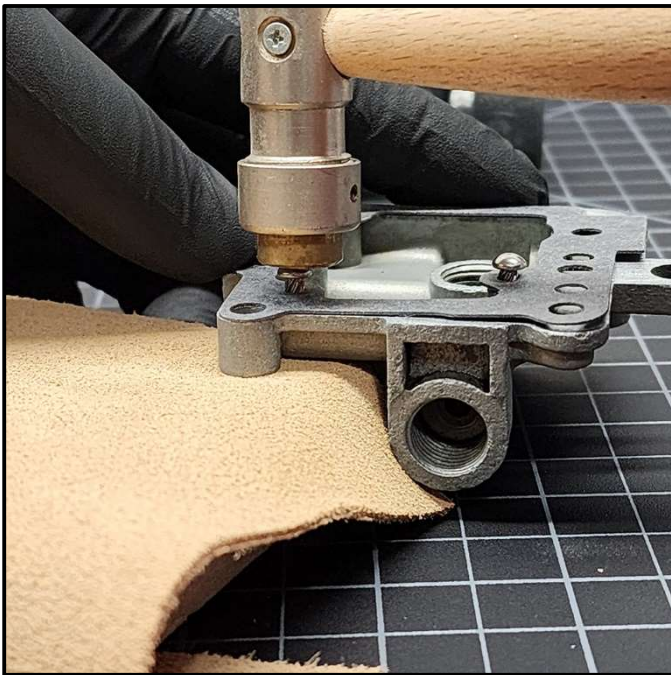
Figure 16 – Using a piece of 0.5” pine board wrapped with leather, the first hammer drive screw is driven into the float chamber cover. The wood and leather will prevent the force of the hammer from warping the soft metal of the float chamber cover during this step.
