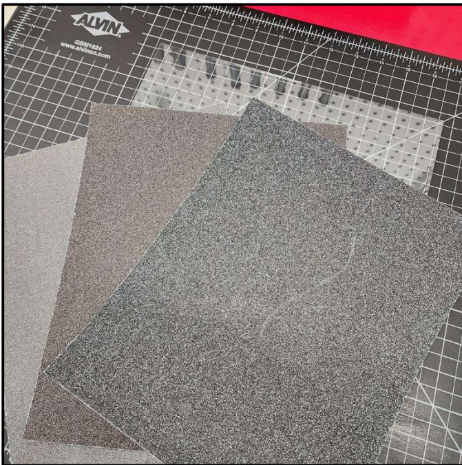
Figure 7 – To plane a small mating surface by hand, a piece of glass offers an ideal smooth surface. Three grits of emery cloth are required; coarse (50 grit), medium (80 grit), and fine (150 grit).
