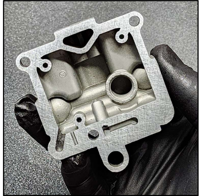
Figure 10 – The coarse emery cloth has flattened the mating surface, as there is evidence of sanding on the entire surface. It is now ready for the medium grit emery cloth.
