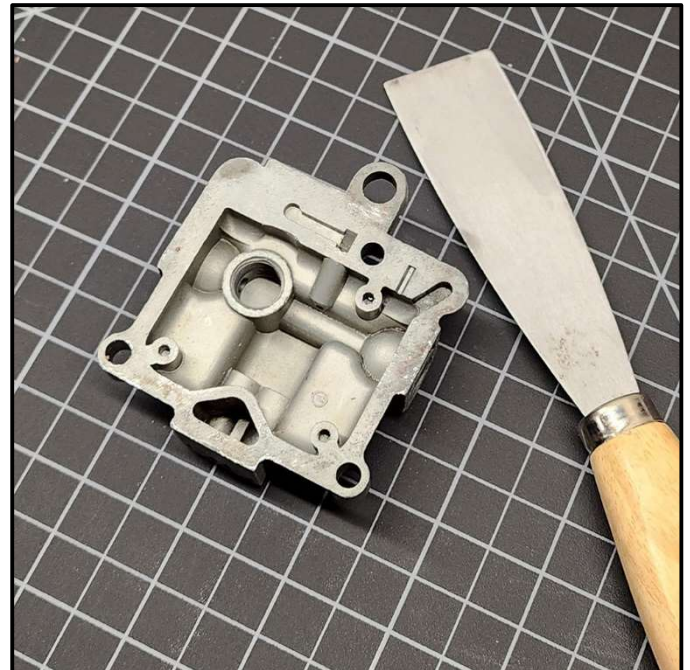
Figure 5 – The scraper effectively cleaned off the RTV material without damaging the mating surface of the float chamber cover.
