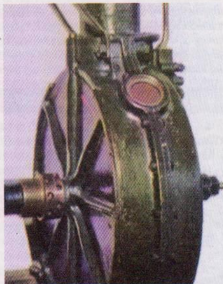
Daimler's Einspur engine may have had the first crankcase breather in 1885.
